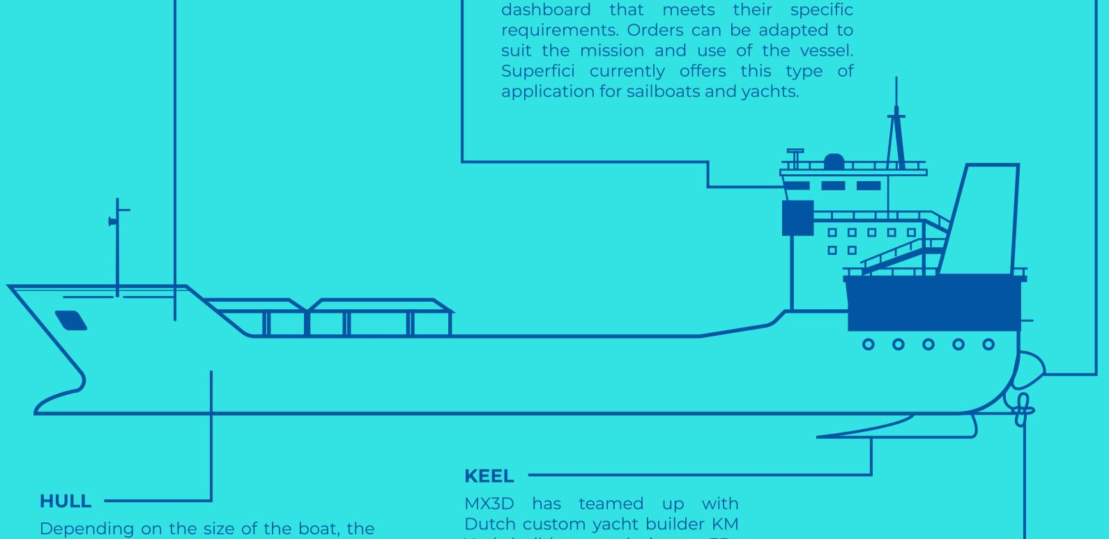
Depending on the size of the boat, the hull can be made using 3D printing, in particular with composite and recycled materials. Among other things, this minimizes assembly steps. For example, Caracol designed the hull of the Beluga sailboat, all in one piece from recycled polypropylene containing 30% glass fibers. MX3D has teamed up with Dutch custom yacht builder KM Yachtbuilders to design a 3Dprinted aluminum keel. The keel, made using WAAM technology, is 4 meters long and 650 mm in diameter.
